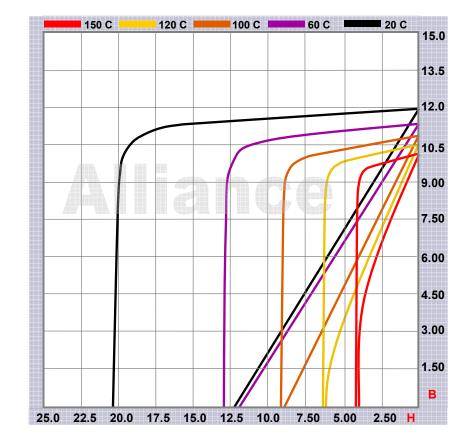
**Typical Minimum** G **Residual Induction Br** 12,000 11,700 11,500 11,000 **Coercive Force Hc** Oe **Intrinsic Coercive Force Hci** Oe 22,000 20,000 35 MGOe 33 Max. Energy Product (BH)max Lb/in3 .2673 **Material Density** С 150 Max. Operating Temperature **Temperature Coefficient for B** -%/C 0.11 -%/C **Temperature Coefficient for H** 0.60 Oe **Required Magnetizing Force** 60,000 Nd, B, Fe, Dy, Co **Material Composition**
