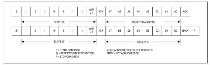
Figure 10. Reading One Byte of Data from MAX30102
