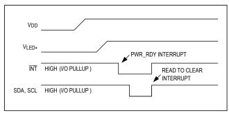
Figure 6. Power-Up Sequence of the Power Supply Rails
