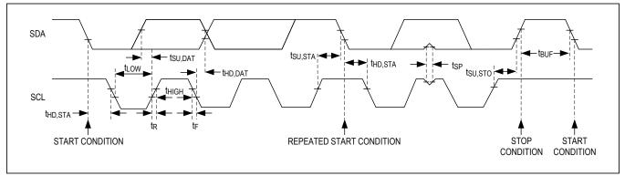
Figure 1. I<sup>2</sup>C-Compatible Interface Timing Diagram
