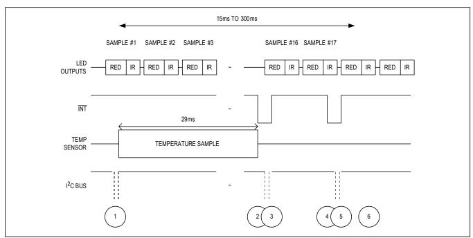
Figure 4. Timing for Data Acquisition and Communication When in SpO<sub>2</sub> Mode
