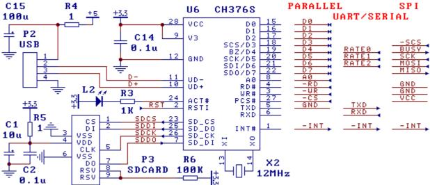
This is 3.3V or 3V supply voltage CH376 operations USB Flash Drive and SD card application circuit. P3 is simplify SD card slot, SD card plug status pin can directly connected to the MCU I/O or interrupt input pin.
